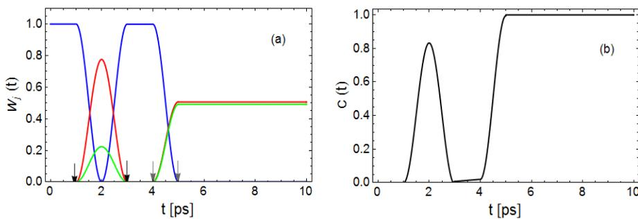
**Figure 2.** Evolution of the level populations  $W_j$  of two coupled qubits in the recording of Bell states (a) and the dynamic of the concurrence  $C(t)$  (b). The blue curve characterizes the behavior of  $W_1(t)$ , the red curve –  $W_2(t)$ , the green –  $W_3(t)$ , the black –  $W_4(t)$ .
